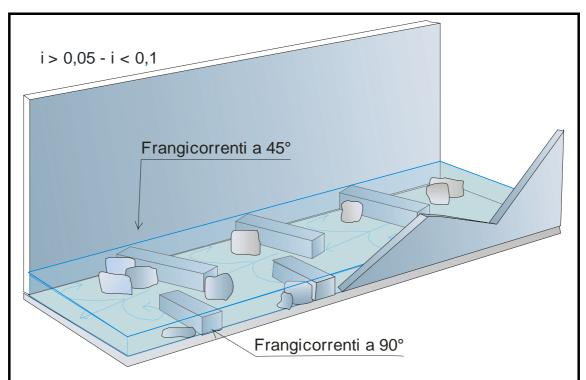
**Fig. 22.12** - Passaggio a rallentamento (Da *Ontario's Stream Rehabilitation Manual*, Ontario Streams, modif.).
